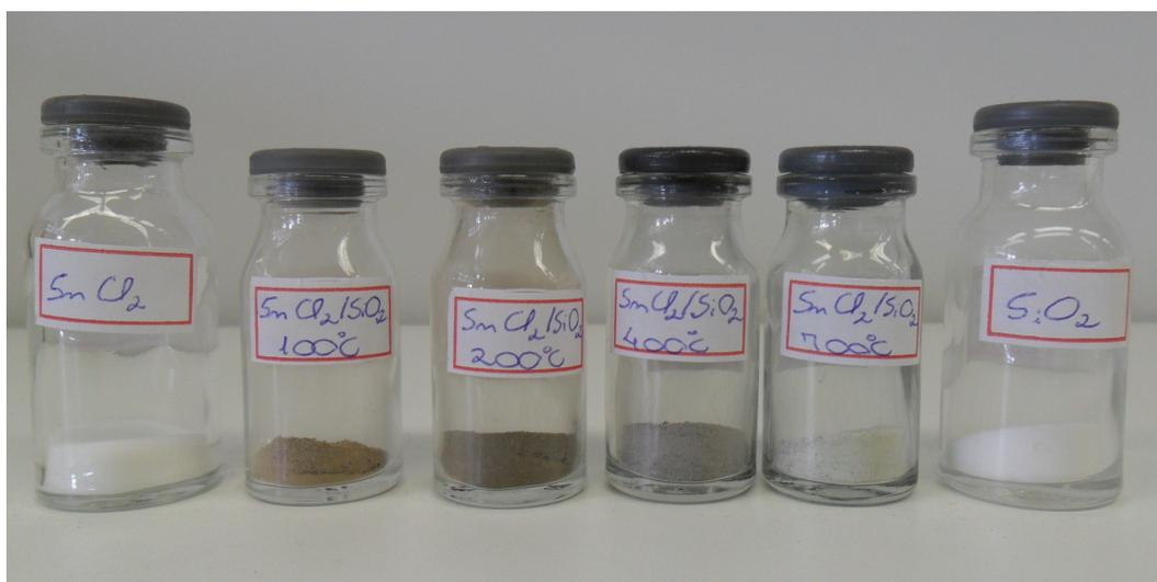
Figura 4. Foto do  $\text{SnCl}_2$ ,  $\text{SnCl}_2/\text{SiO}_2(100^\circ\text{C})$ ,  $\text{SnCl}_2/\text{SiO}_2(200^\circ\text{C})$ ,  $\text{SnCl}_2/\text{SiO}_2(400^\circ\text{C})$ ,  $\text{SnCl}_2/\text{SiO}_2(700^\circ\text{C})$  e  $\text{SiO}_2$ , respectivamente.
