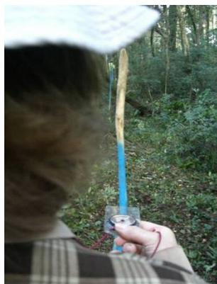
FIGURA 2 – DEMARCAÇÃO DAS TRILHAS COM AUXÍLIO DE BÚSSOLA E ESTACAS
