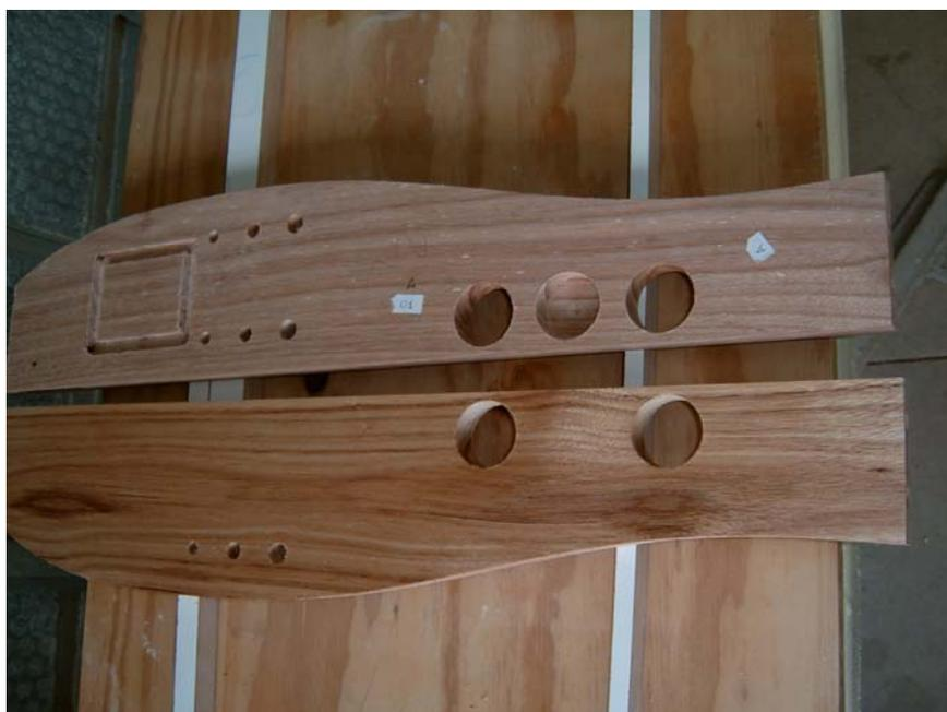
FIGURA 19 – CORPOS-DE-PROVA COM UMA DAS FACES COM ACABAMENTO SUPERFICIAL
