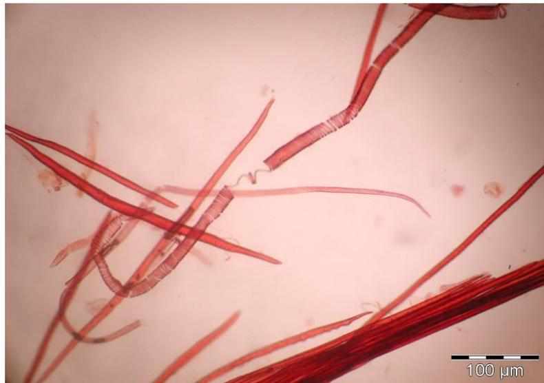
FIGURA 33 – DETALHE DOS ELEMENTOS EM ESPIRAL DE CELULOSE PRESENTES NAS FIBRAS DE COCO
