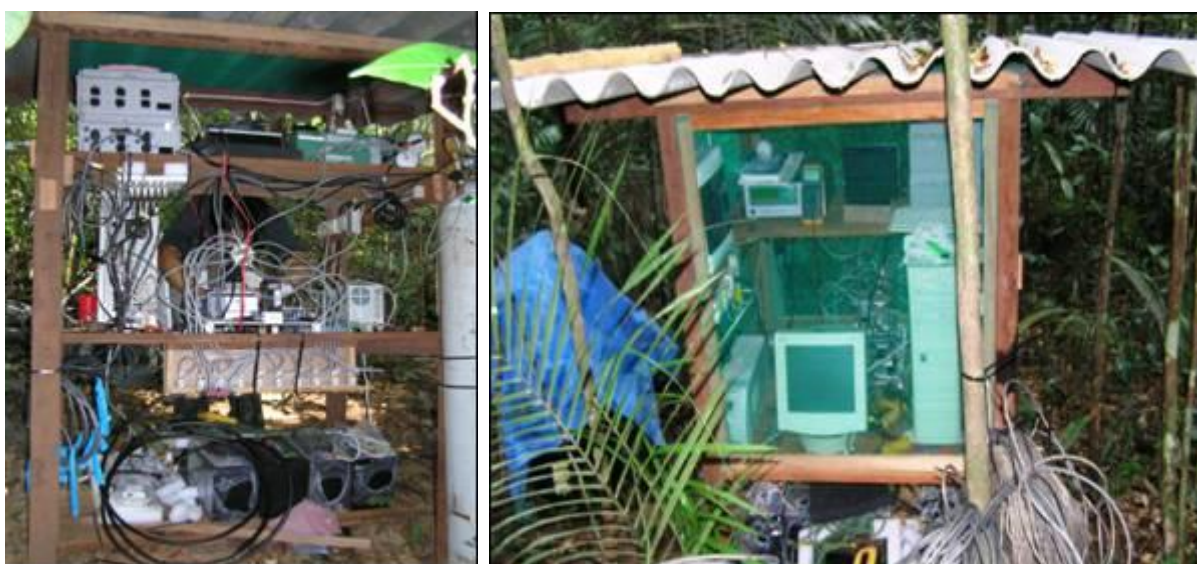
Figure 3: Draino measurement system used in Manaus LBA (South Face, see also Figure 4).
