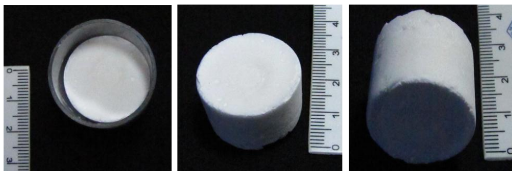
Figure 1. Macro structures of cellulose aerogels regenerated after freeze-drying. Left: cylindrical mold used during freeze-drying.
